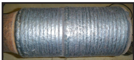
Re-built Tool Joint prior to machining
