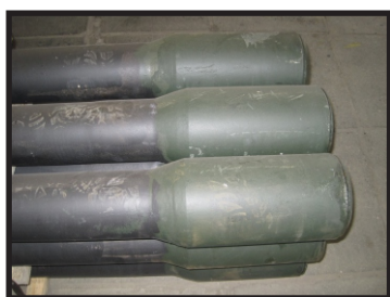
Re-built Tool Joints after machining
