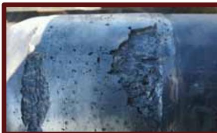
Sharp edges, trapped sand, or other imbedded debris affect the “casing friendliness” of cracked or spalling hardbands
