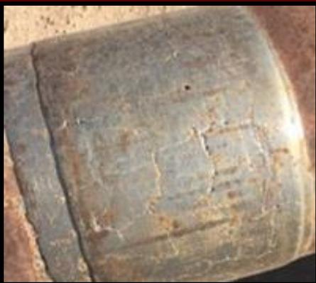
The photos above are two examples of hardbands exhibiting unacceptable cracking. Hardbanding in this condition should never have new hardbanding re-applied over them. It must be ground out and rebuilt before new hardbanding can be applied.
